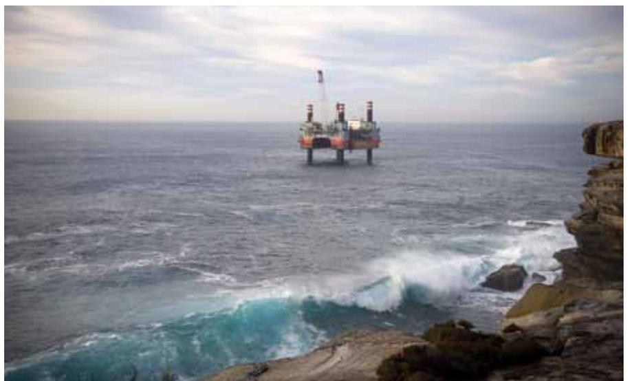
**A jack-up barge, Seafox 6, was used as a drilling platform for the inlet and outlet shafts for the desalination plant. Construction of the plant was completed on time and under budget.**
